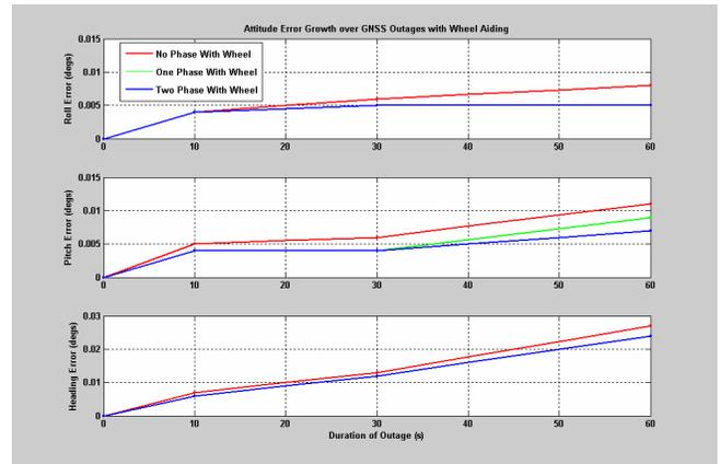
Figure 13 Attitude Error Growth Over GNSS Outages with Wheel Sensor Aiding
