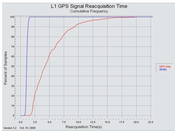
Fig. 4. L1 Signal Reacquisition Histogram
