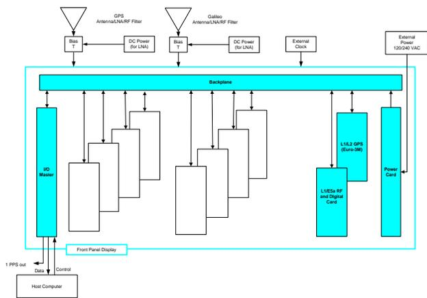
**Figure 2:** Block Diagram of GTR
