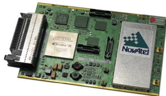
Figure 1: Galileo L1/E5a Receiver Card
