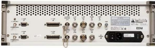
**Figure 6:** GUS Signal Generator Back Panel
