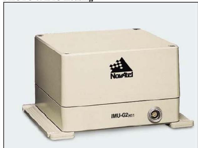
The SiIMU-01 is connected to the OEM4-G2 via an RS-232 serial interface. Serial messages are transmitted at a 100 Hz rate from the IMU to the OEM4-G2. The first byte in each serial message triggers an interrupt serviced by a timing function tightly bound to the receiver's correlator chip. The time tag generated is accurate to 10 microseconds. The time tag is buffered while the rest of the 10 msec serial message is accumulated.
