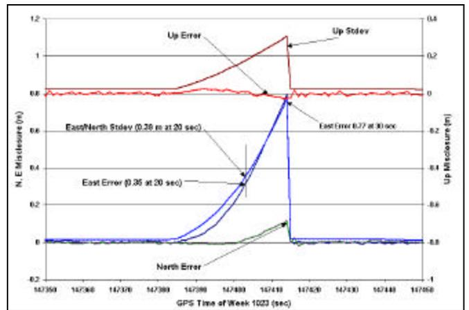
**Figure 4: Detail 30 sec Open Loop Error**
