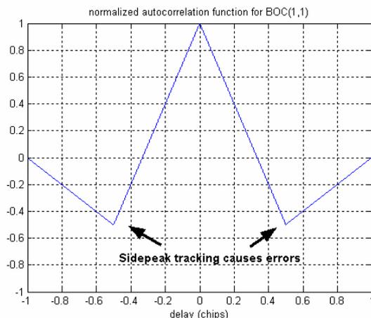
Figure 11 BOC(1,1) Correlation Function - Multiple Tracking Points
