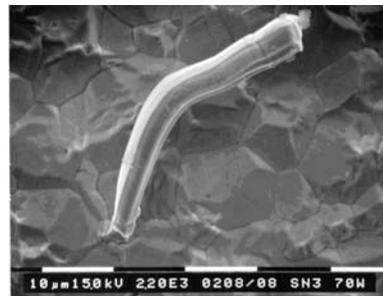
*Tin whisker electron micrograph, showing the behaviour of the filament to grow at right angles to the plated surface. Photograph courtesy of EFSOT (Environmentally Friendly Soldering Technologies), [www.efsot-europe.info](http://www.efsot-europe.info)*
