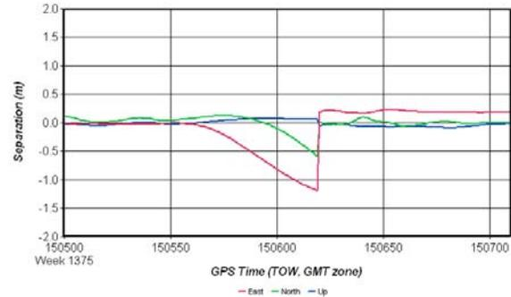
Figure 2: Forward direction error with loosely coupled processing
