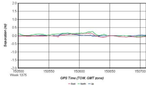
Figure 3: Forward direction error with tightly coupled processing
