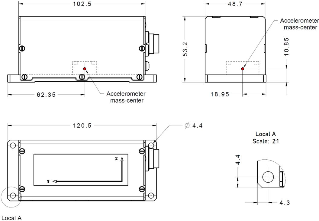
DIMENSIONS ARE IN MILLIMETERS
