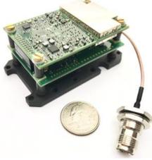
The Inertial Labs **INS-B-OEM** utilizes advanced single antenna GNSS receiver, barometer, 3-axes each of calibrated in full operational temperature range Advanced MEMS Accelerometers and Gyroscopes to provide accurate Position, Velocity, Heading, Pitch and Roll of the device under measure. **INS-B-OEM** contains Inertial Labs new on-board sensors fusion filter, state of the art navigation and guidance algorithms and calibration software.
